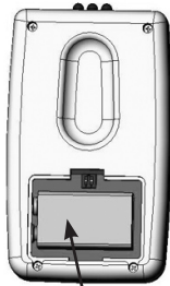
9V battery (access panel removed)
