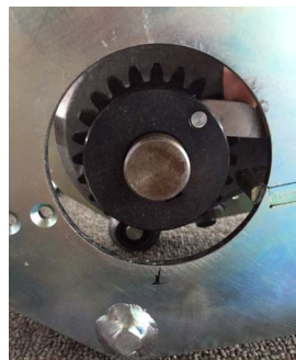
Side view of brake dog flipped up (engaged)
