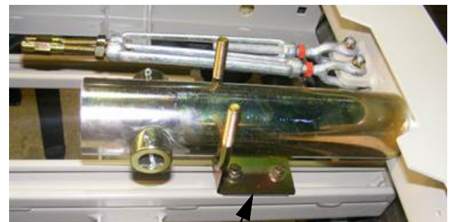
Figure 6 Add/remove shims behind cylinder bracket
