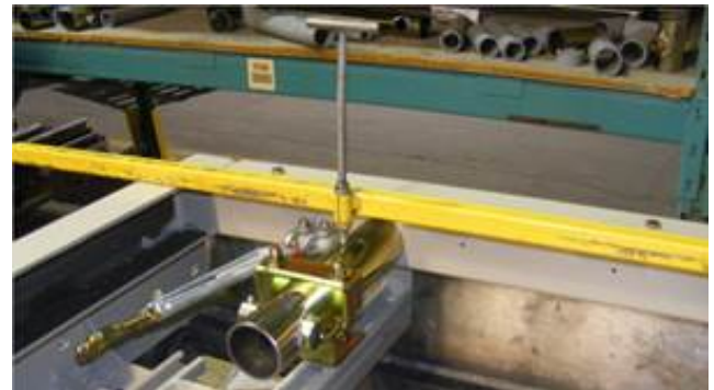
Figure 5 Check distance between level and pillar
