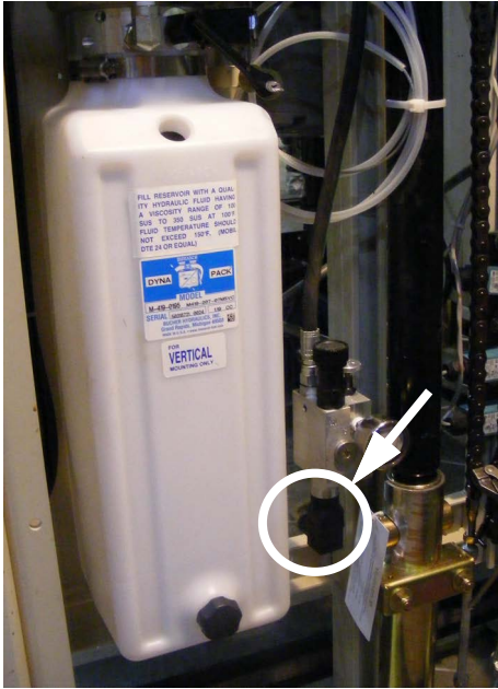
Figure 48 Location of pressure switch
